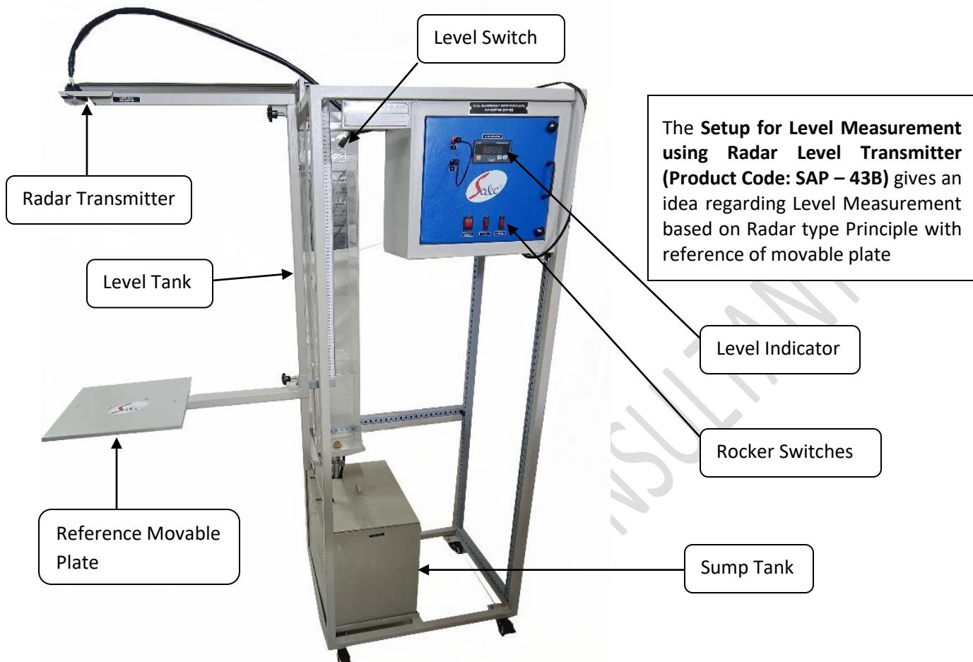
**LEVEL MEASUREMENT USING RADAR LEVEL TRANSMITTER (SAP – 43B)**
